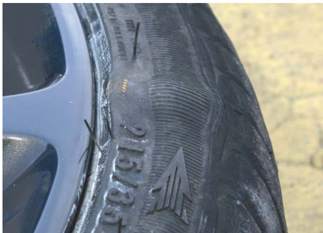
Bulges or eggs in the sidewall show the rubber has started to deteriorate and the tyre must be replaced
