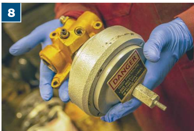
One of the car's rebuilt accumulator spheres, featuring all gaskets, a full charge of nitrogen and a rebuilt valve body
