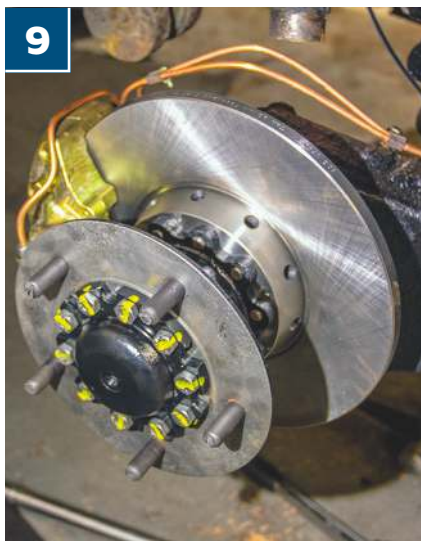
One of the reconditioned rear hub assemblies, with new brake lines, calipers and new brake discs also bolted in place
