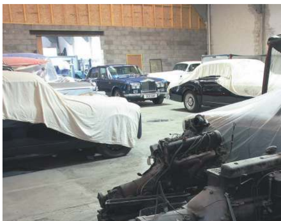
Long-term storage can result in tyres developing flat spots, even if they remain correctly inflated
