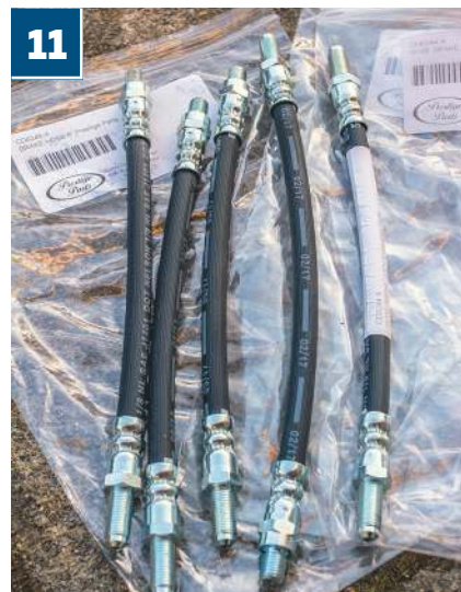
We're going flexi-hose crazy! In this photo, you can see the rear brake caliper hoses and suspension height control pipework
