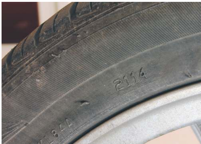
The four-digit date code 2114 means this tyre was manufactured in the 21st week of 2014
