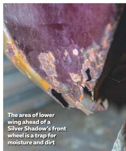
The Silver Shadow was the first Rolls-Royce with monocoque construction, which brings its own rust issues
