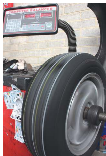
Balancing a wheel adds weights to the inside rim to help eliminate unwanted vibrations through the steering and chassis
