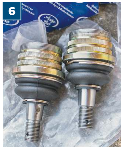
Fresh chassis equipment, including these top ball joints and their housing assemblies, eliminated negative suspension and steering feedback
