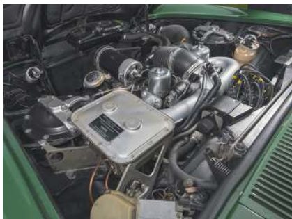
The Silver Shadow and T-series used the L-series V8 in 6230cc guise until 1970
