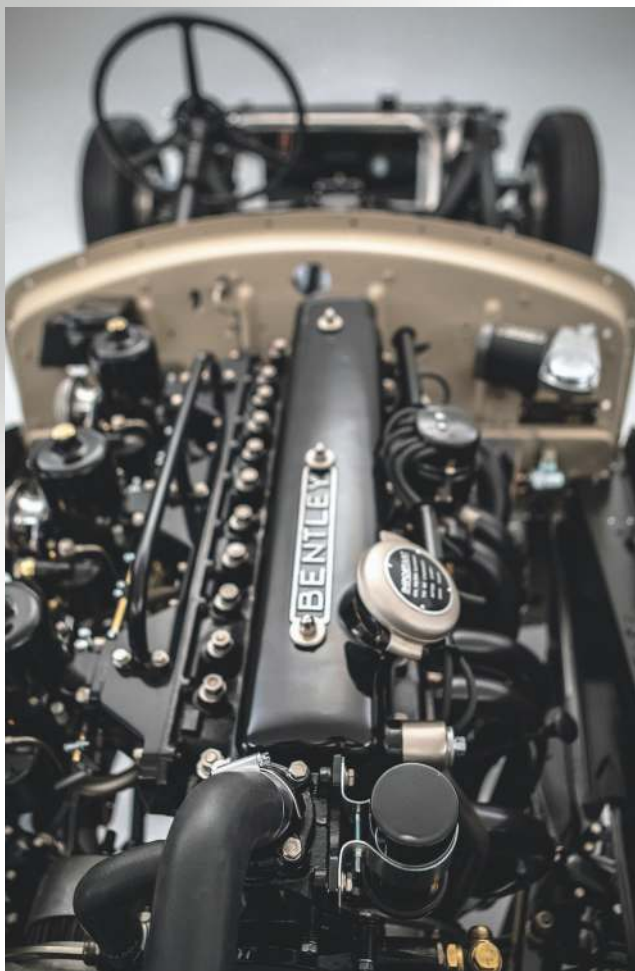
The Blizzard employs a usefully updated R-Type powerplant
